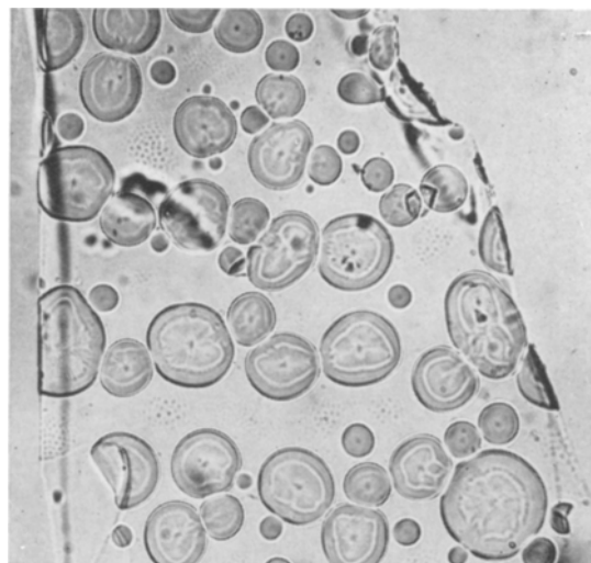
Figure 8 Surface fragment of borosilicate glass (one hundred exposures at 7 kV, 400° C) mounted in liquid of refractive index 1.474 showing second-phase regions; transmitted light. ( \times 130 )
